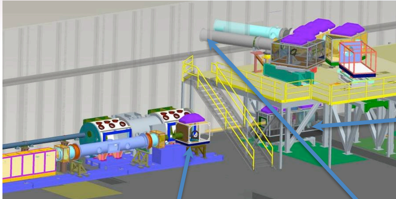
Schematic of main amps and transport of the Z-Petawatt laser
